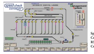
Speed Check Conveyor RMS Computer Control System
